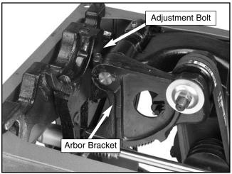
Figure 22. Arbor bracket adjustment locations.
